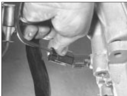
5.14c . . . and the reversing light switch
