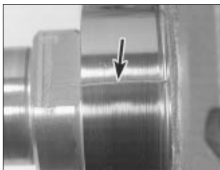
17.11 Lay the Plastigauge strips (arrowed) on the main bearing journals, parallel to the crankshaft centre-line
