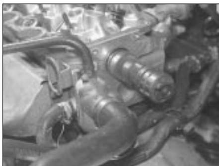
11.12 Withdraw the camshaft from the cylinder head
