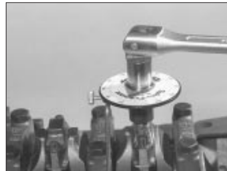
18.11 Angle-tightening the big-end bolts using the correct tool
