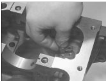
13.1a Unbolt blanking plugs (where fitted) to clean out oilways . . .
