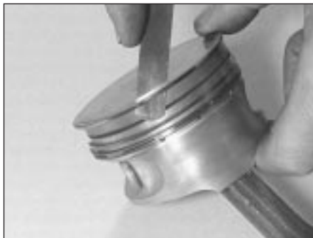
11.14 Using feeler gauge blades to remove piston rings
