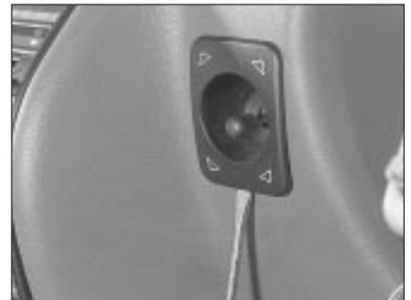
24.2 Carefully prise the speaker balance control joystick from its location
