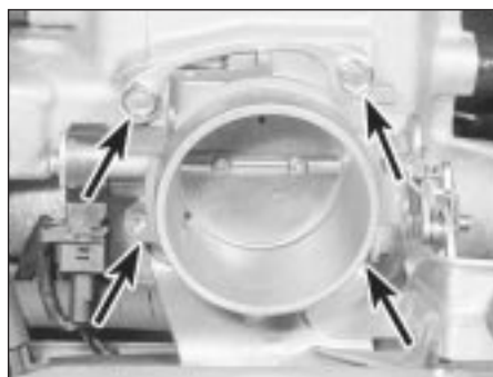
14.7 Throttle housing retaining bolt locations (arrowed)
