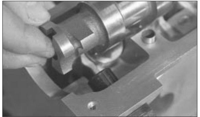
11.5b Inlet camshaft has lobe for camshaft position sensor
