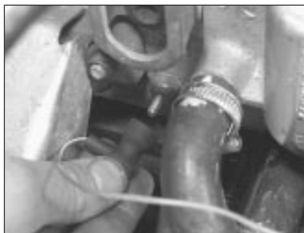
4.12a Disconnect the wiring at the temperature gauge sender unit . . .
