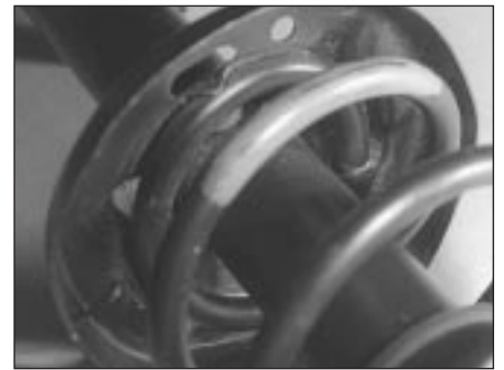
5.9 Correct spring location in its lower seat
