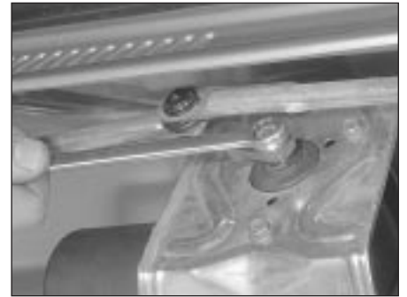
16.7 Unscrew the nut from the wiper motor driving shaft
