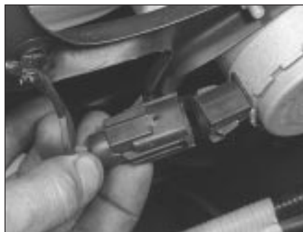
5.5 Disconnecting the multi-plug from the radiator cooling fan motor
