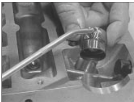
11.17 Oil liberally when refitting hydraulic tappets
