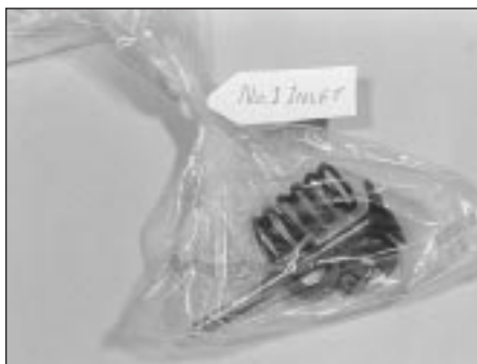
7.9 Use a labelled plastic bag to store and identify valve components
