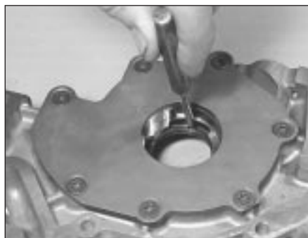
15.2 Driving out crankshaft right-hand oil seal
