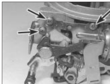
24.5 Undo the three screws securing the choke mechanism (arrowed)
