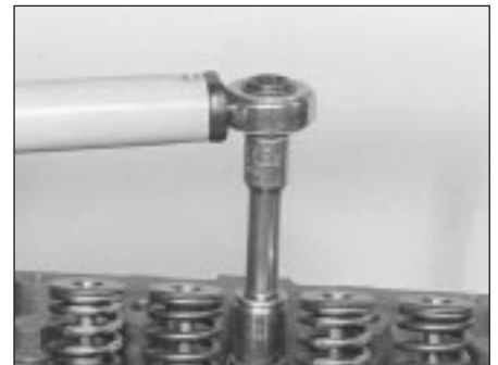
7.27b Tightening the cylinder head bolts (Stage 1)
