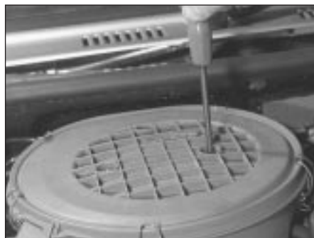
2.3 Undoing the air cleaner retaining screws (HCS engine shown)
