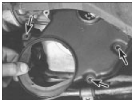
7.11 Removing timing belt lower cover - bolt locations arrowed
