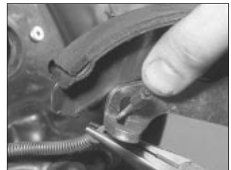
6.5 Disengage the handbrake cable from its operating lever on the trailing shoe
