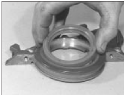
14.11a Positioning the crankshaft rear oil seal in its housing
