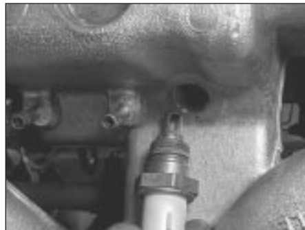
14.44 Removing the intake air temperature sensor from the rear of the inlet manifold (Zetec engine shown)
