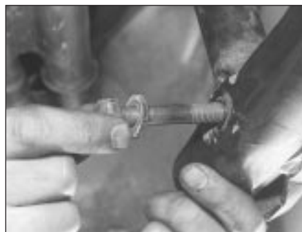
10.3 Lower suspension strut-to-axle mounting bolt
