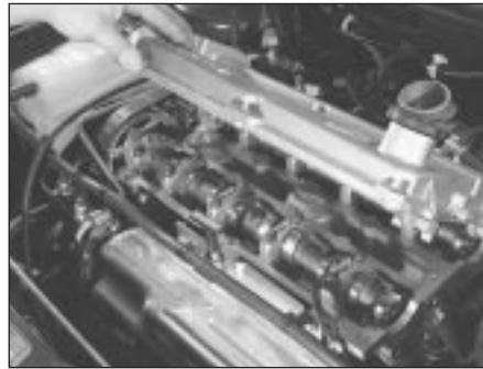
4.8 Removing cylinder head cover
