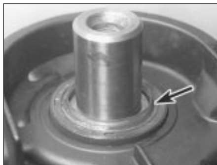
14.9b With the oil pump refitted, remove the protective guide (arrowed)
