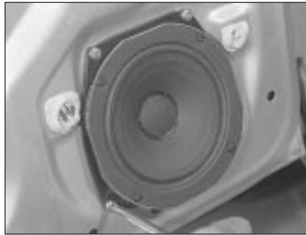
23.3 Remove the screws securing the speaker assembly to the front door
