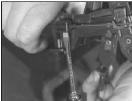
11.7a Releasing outer cable clamping cover ...
