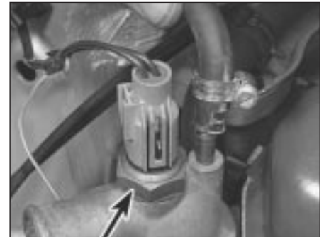
4.4b Disconnecting the expansion tank top hose from the thermostat housing (HCS engine). Radiator cooling fan thermal switch (arrowed)
