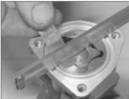
13.4c Checking the rotor endfloat
