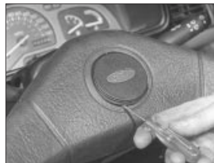
19.2 Removing the motif from the steering wheel
