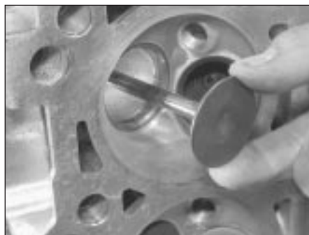
9.9 Insert the valve into its guide
