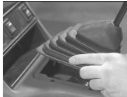
45.3 Removing the gear lever gaiter from the centre console
