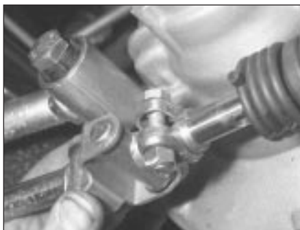
5.24a Disconnect the gearchange linkage . . .
