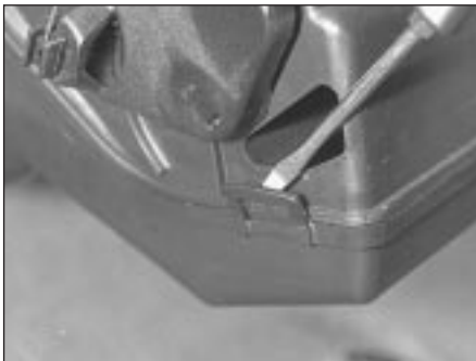
11.28a Unclipping the lower heater casing cover
