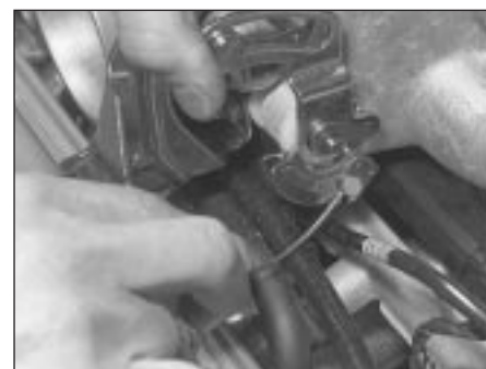
5.45 Accelerator cable retention arrangement at the throttle linkage
