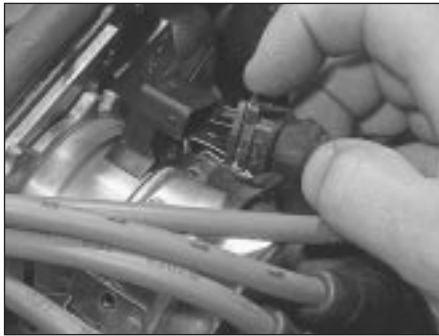
7.4a Disconnecting the distributor multi-plug
