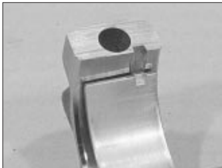
18.3 Tab on each big-end bearing shell must engage with notch in connecting rod or cap
