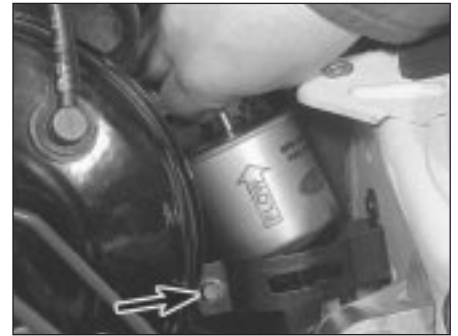
30.6b Removing the bulkhead mounted fuel filter. Clamp bolt (arrowed)
