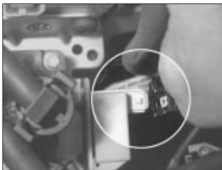
5.14a Disconnect the wiring multi-plug from the ignition coil . . .
