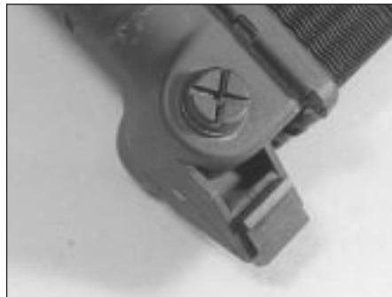
23.3 Drain plug location at the base of the radiator - use a coin to unscrew the plug
