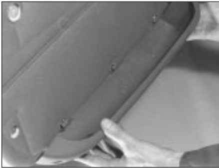
21.5 Disengaging the hook fixings on the base of the door stowage pocket/speaker grille moulding
