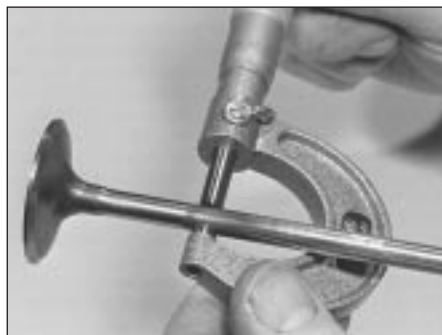
8.12 Measuring the diameter of a valve stem
