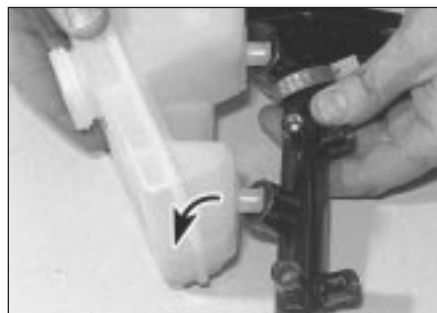
9.5 Removing the brake fluid reservoir from its seals in the master cylinder
