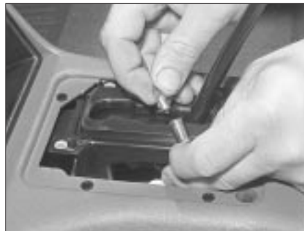
6.3b . . . followed by the (bayonet fitting) bulb
