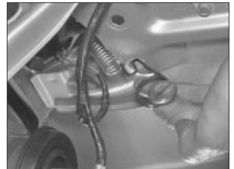
7.7a Release the front direction indicator light retaining spring from its body location . . .
