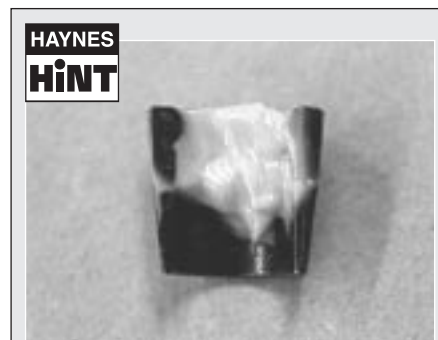
A little grease applied to the collet groove will help retain them in position.
