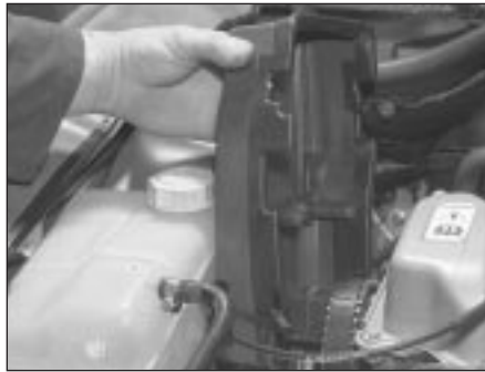
7.3 Upper timing belt cover removal
