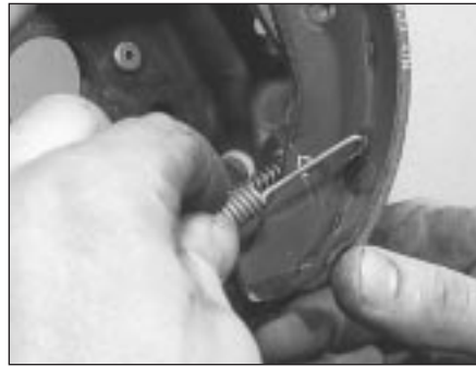
6.4a Detach the lower pull-off spring
