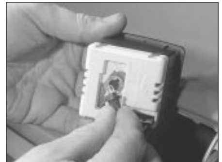
6.8 Withdrawing the clock illumination bulb and its integral holder from the rear of the clock
