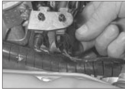
14.28a Release the throttle position sensor multi-plug from its retaining clip and disconnect it
