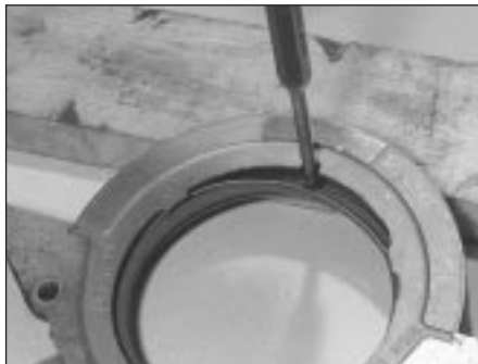
16.18 Rear oil seal removal
