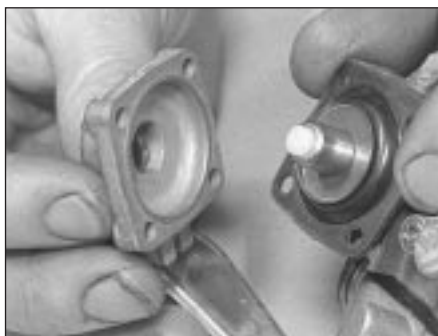
24.11a Remove the accelerator pump cover ...
