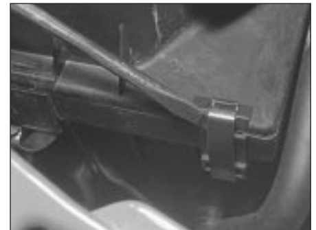
24.6 On EFI fuel injection engines, release the retaining clips and lift off the air cleaner lid
