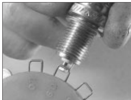
21.12b Spark plug manufacturers recommend using a wire-type gauge when checking the gap - if the wire or feeler gauge does not slide between the electrodes with a slight drag, adjustment is required
