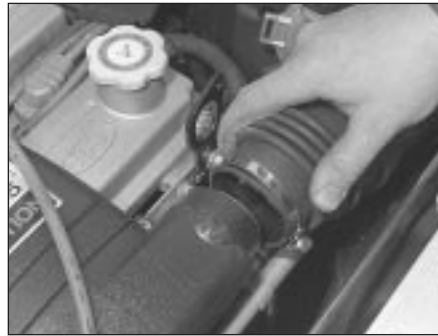
24.8 . . . slacken the hose clip and disconnect the intake hose from the air intake duct . . .
