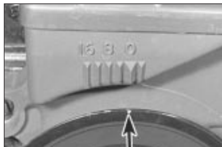
3.6a Crankshaft pulley notch (arrowed) aligned with the TDC (0) mark on the timing belt cover
