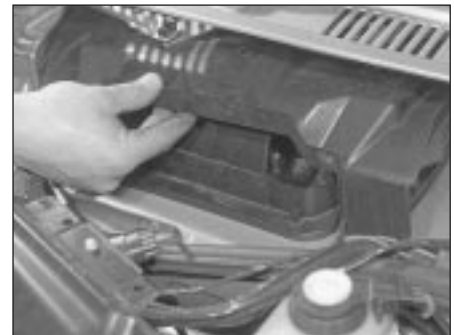
11.16 Removing the cover from the heater fan motor assembly
