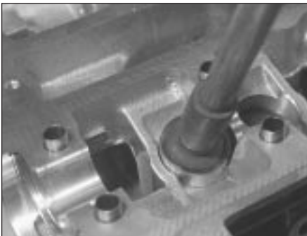
11.6a Removing hydraulic tappets
