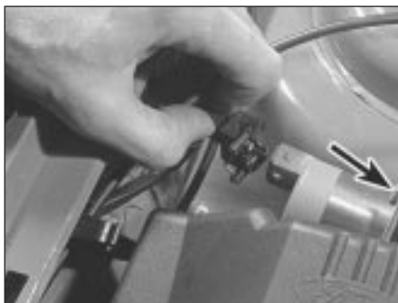
14.24 Disconnect the multi-plug from the idle speed control valve. Upper valve retaining bolt (arrowed)
