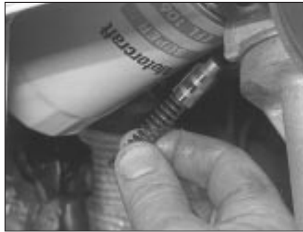
14.9b . . . to withdraw oil pressure relief valve spring and plunger
