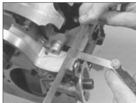
14.13 Oil pump must be positioned accurately
