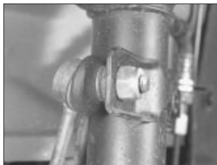
6.3 Anti-roll bar connecting link-to-strut connection
