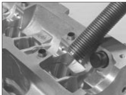
7.21b . . . can be replaced by home-made tool if suitable spring can be found
