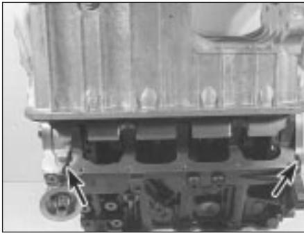
13.13a Apply sealant (arrowed) as directed when refitting sump
