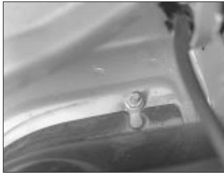
16.6b . . . then disengage the right-hand half of the panel from under its single retaining nut (left-hand shown)
