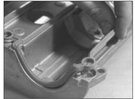
4.10 Ensure gasket is located correctly in cover groove
