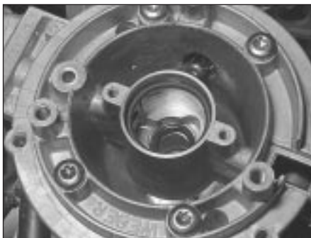
14.5d Injector seals in the CFI unit
