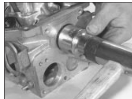
11.22 Driving a new blanking plug into position
