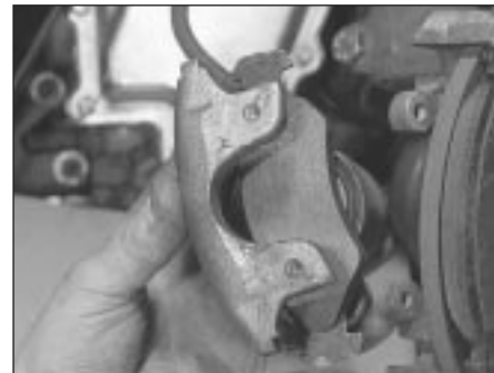
2.3b . . . unscrew the bolts then withdraw the caliper from the anchor bracket
