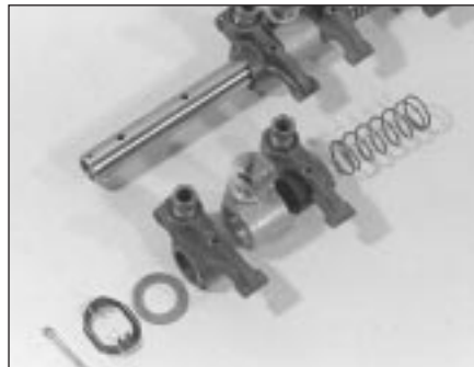
6.4 Rocker shaft partially dismantled for inspection
