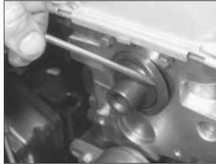
10.2 Camshaft front oil seal removal
