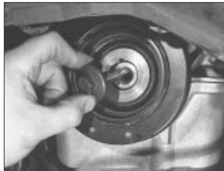
6.9 Unscrew pulley bolt to release crankshaft pulley
