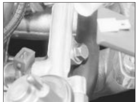
14.12a Remove the fuel rail retaining bolts ...
