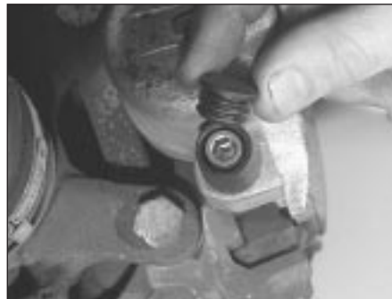
2.3a Remove the rubber blanking plugs for access to the caliper mounting bolts . . .
