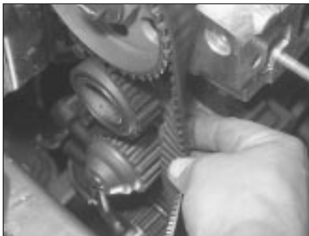
8.13 Checking the tension of the timing belt
