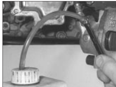
13.22 Bleeding the hydraulic system using a one-way valve kit
