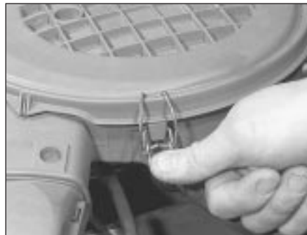
24.3 . . . then spring back the clips and lift of the lid
