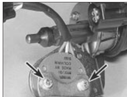
14.45 Throttle position sensor retaining screws (arrowed) (shown with throttle plate control motor removed)
