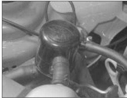
25.5 Crankcase ventilation system filter on CVH engines
