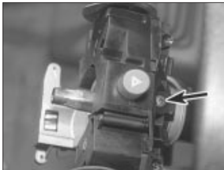
20.5 Steering column multi-function switch retaining screw (arrowed) (steering wheel removed for clarity)
