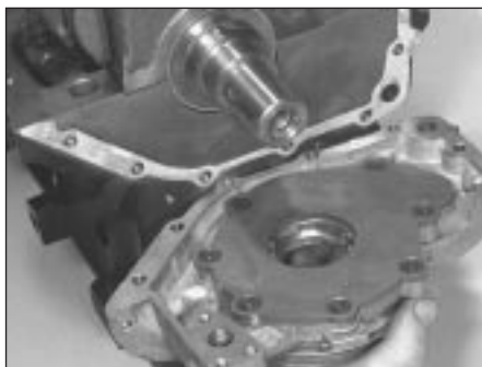
14.9a Refit the oil pump
