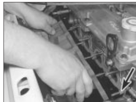
3.18 Fit a new plastic guide sleeve to the stud (arrowed) when refitting the manifold (Zetec engine models)
