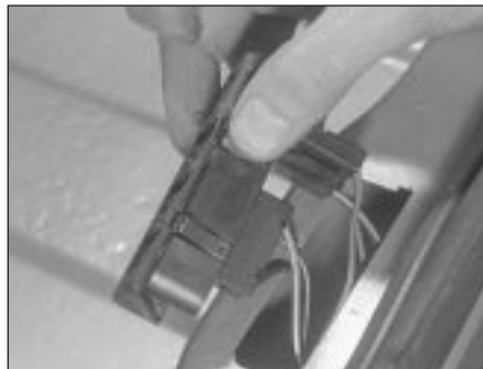
4.46 Withdrawing the luggage area contact plate for access to disconnect the multi-plug
