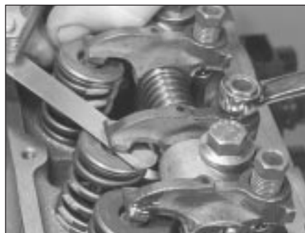
5.6 Adjusting the valve clearances
