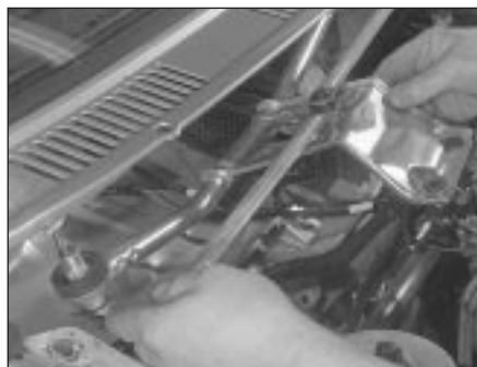
17.4 Removing the wiper motor bracket and linkage assembly (wiper motor removed)
