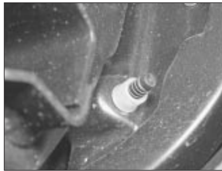
27.3 Handbrake adjustment plunger located on the inside face of each rear brake backplate
