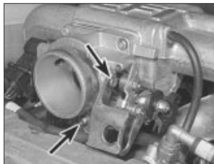
14.5 Unscrew the retaining bolts (arrowed), and detach the accelerator cable support bracket
