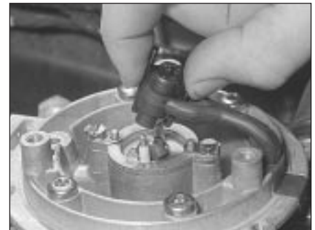
14.4 Disconnect the multi-plug from the injector
