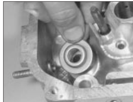
9.7 Fit the lower retainer
