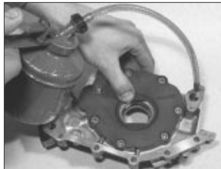
14.8 Prime the oil pump prior to fitting
