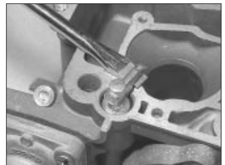
24.10 Carefully prising out the accelerator pump discharge tube assembly
