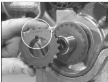
9.8 "FRONT" marking on outside face of crankshaft toothed pulley - note which way round thrustwasher behind is fitted
