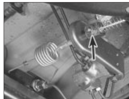
22.3 Light-laden valve linkage adjustment locknut (arrowed)
