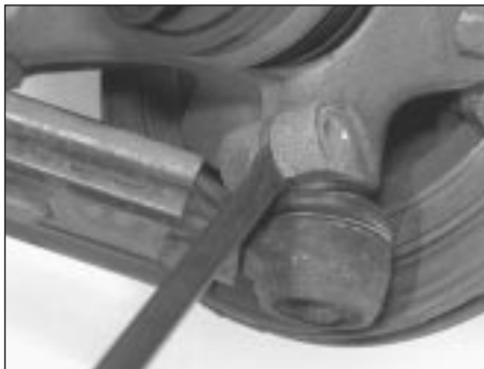
2.11b . . . prise open the joint . . .
