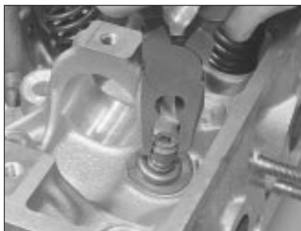
7.14 Prise off the valve stem oil seal
