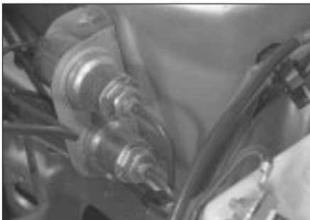
20.1a Pressure control valves located on left-hand inner wing panel
