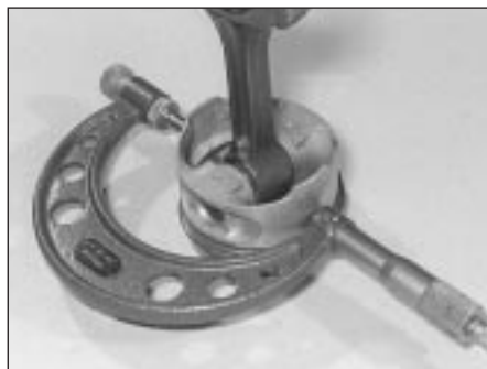
13.13 Measure the piston skirt diameter at right-angles to the gudgeon pin axis, just above the base of the skirt
