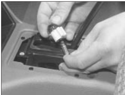
6.3a Remove the selector illumination bulb cover . . .
