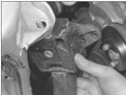
15.10 Undo the three bolts securing the mounting assembly to the cylinder block and withdraw the mounting
