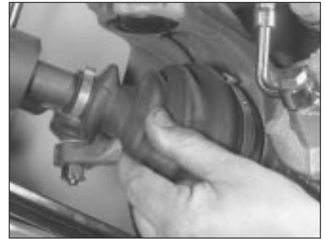
11.2 Check the driveshaft gaiters by hand for cracks and/or leaking grease
