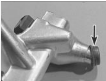
14.20 Fit new nose seals (arrowed) before refitting the fuel rail
