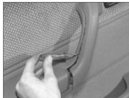
21.4a Detaching armrest/doorpull removable panel
