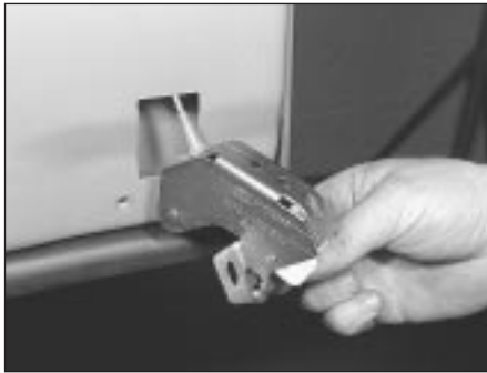
30.12 Courier rear door lower catch removal
