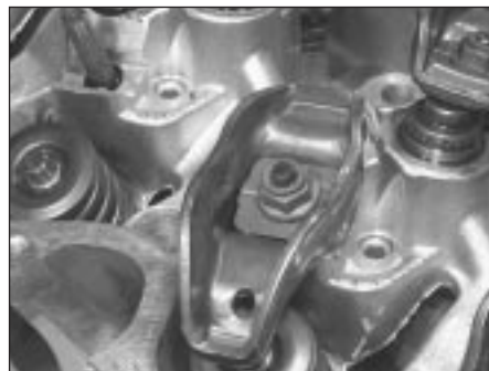
11.5a Undo the rocker arm retaining nut ...
