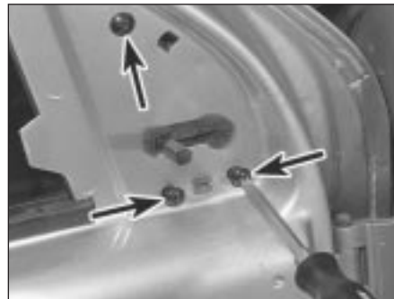
18.8 Removing the three mirror retaining screws (arrowed)
