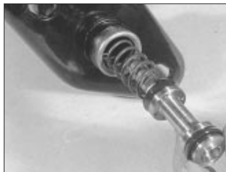
9.8b . . . followed by the secondary piston assembly
