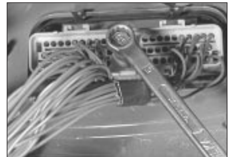
14.36b Undoing the EEC IV engine management module multi-plug retaining bolt
