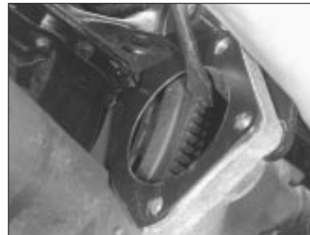
6.6 Using a suitable bar to lock the flywheel ring gear
