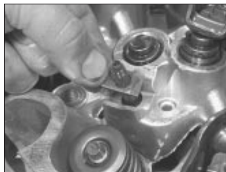
11.5d ... and spacer plate
