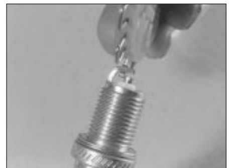
21.13 To change the gap, bend the outer electrode only, and be very careful not to crack or chip the porcelain insulator surrounding the centre electrode
