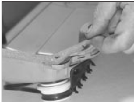
4.8a Fitting a new gasket to the rocker cover
