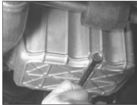
3.7b Removing the engine oil drain plug on the Zetec engine
