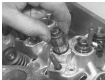
11.6a Removing a hydraulic tappet
