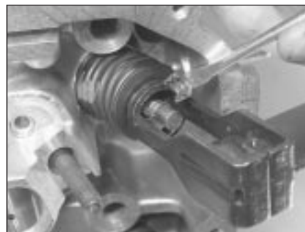
9.11 Insert the split collets into the groove in the valve stem
