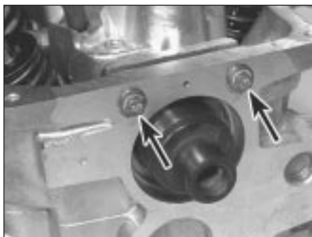
11.10a Undo the two retaining bolts (arrowed) ...
