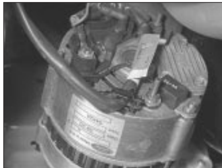
6.10 Wiring loom routing on rear of alternator (CVH engine)
