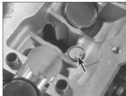
7.23 Cylinder head oil-retaining valve (arrowed)
