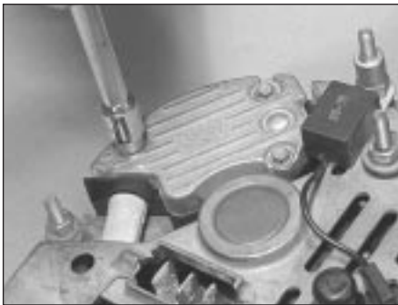
7.7a Removing the regulator and brushbox assembly securing screws (Magneti-Marelli alternator)
