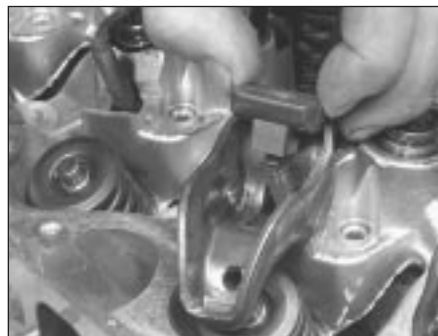
11.5b ... withdraw the guide ...
