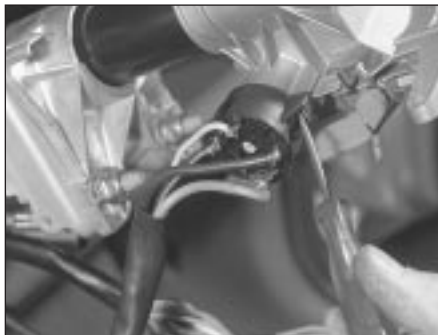
20.6 Removing ignition loom plate from steering column lock housing (steering wheel removed for clarity)
