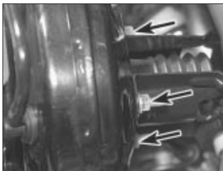
15.6 Nuts securing servo unit to its mounting bracket assembly (arrowed)
