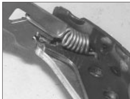
6.7b Detach the adjuster strut
