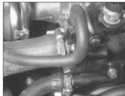
12.13 Disconnect all coolant hoses from thermostat housing
