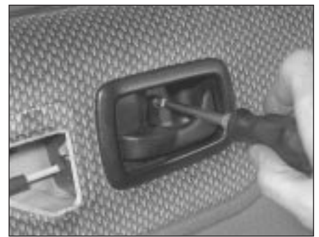
21.2 Removing the door interior release handle bezel (armrest/doorpull shown removed)
