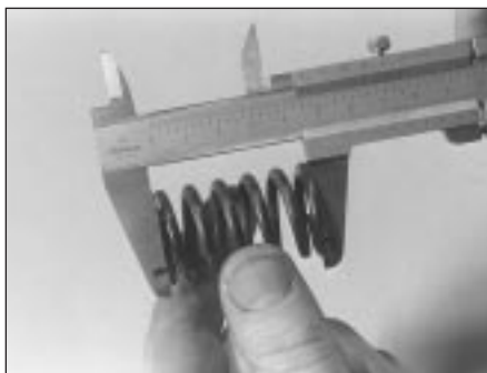
8.18 Checking the valve spring free length
