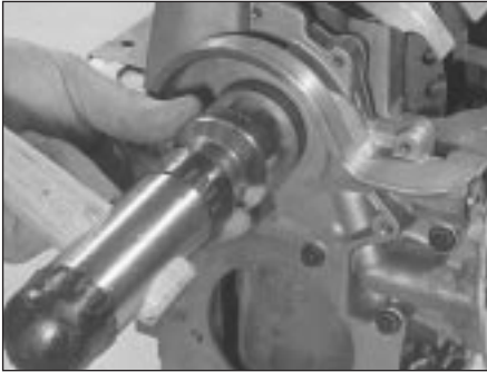
15.6 If seal is tapped into place as shown, exercise great care to prevent seal from being damaged or distorted
