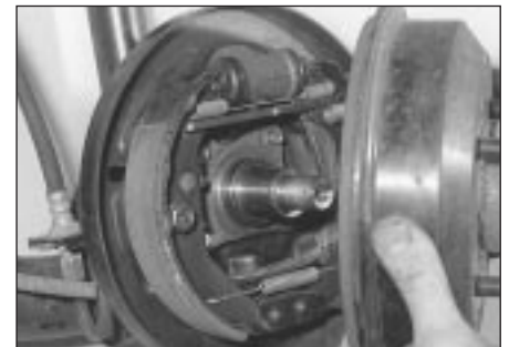
9.5 Slide off the wheel hub/brake drum unit
